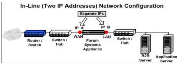
**Figure 3: In-Line Configuration Schematic for Two IP Addresses.**
